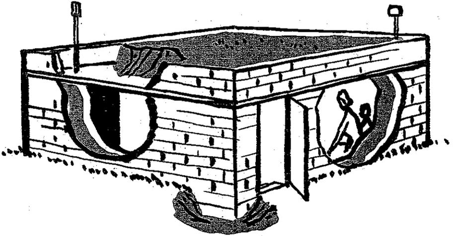
*Aboveground Double-Wall Shelter*, which is a double-walled, concrete block structure with the walls built nearly 2 feet apart. The space between the walls is filled with earth. A roof is built of either poured concrete or wood and covered with earth.
