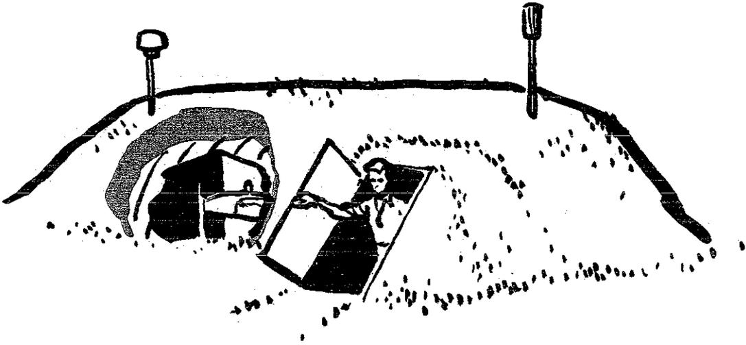
*Preshaped Metal Shelter*, built by placing pre-shaped corrugated metal sections on or close to the surface of the ground and mounding them over with earth.
